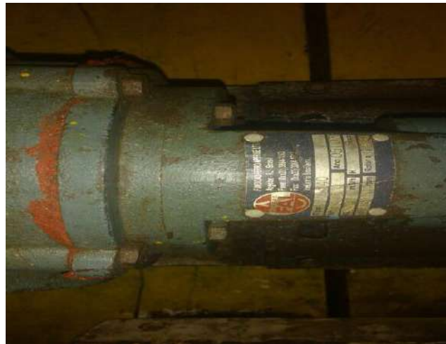
Fig. 2- Centrifugal pump used on the vessel
