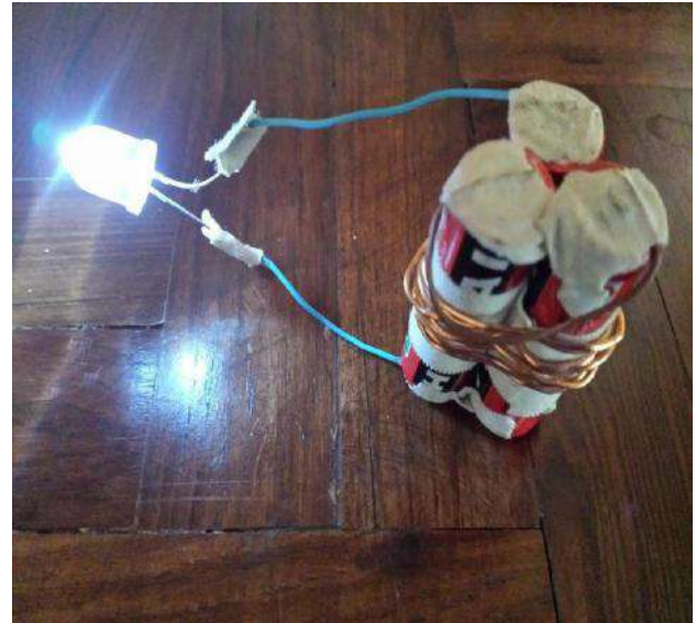
Fig. 31. Direct power supply of an LED by three new batteries of size AA.
