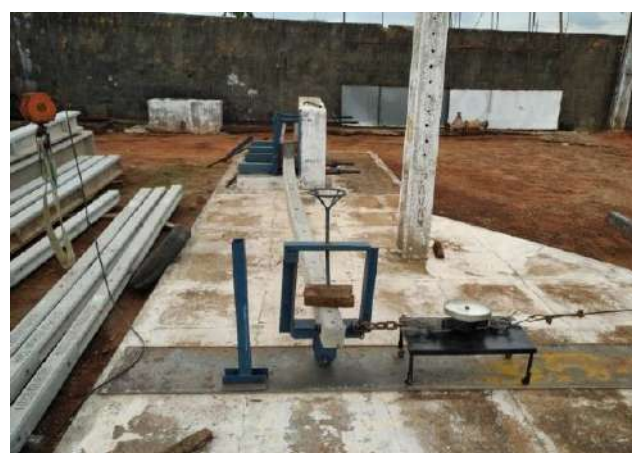
Fig.2: Bending test on molded posts.
