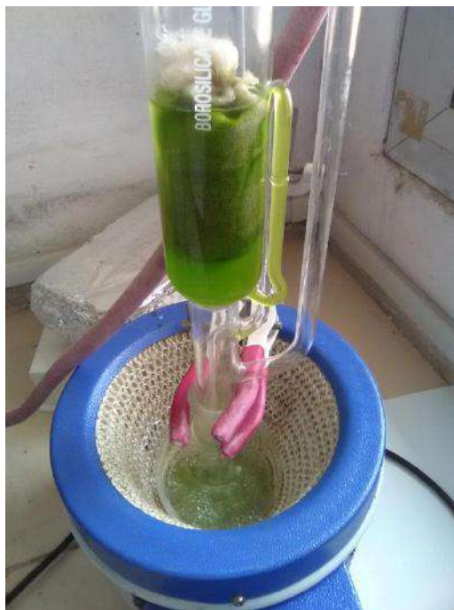
Fig.2: Soxhletion process of sample
