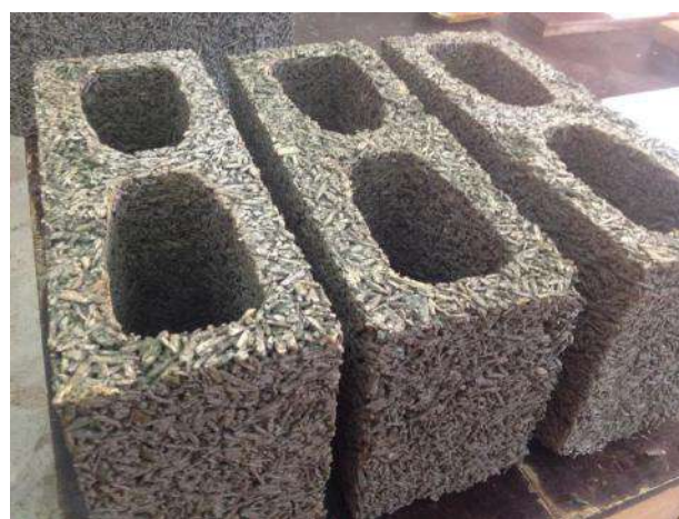
Fig. 1: The cementitious block with wood particles (Villas Bôas, 2016).
