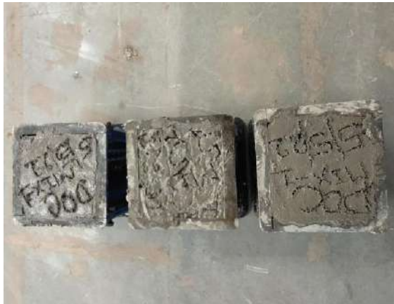
Fig. 3: A typical pervious concrete specimen used in this investigation
