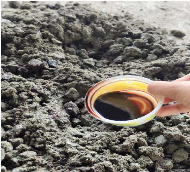
Fig. 2: pervious concrete with super plasticizer
