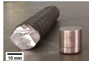
Fig. 4: CA-50 steel bar and cylindrical sample
