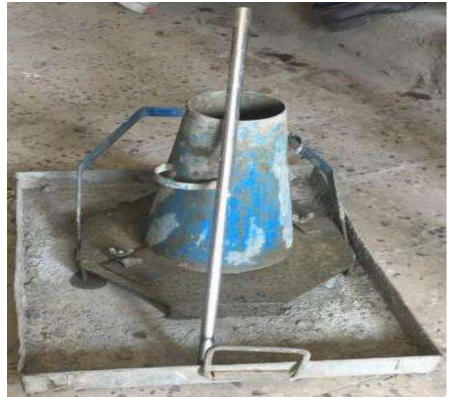
Fig. 4: Slump cone test
