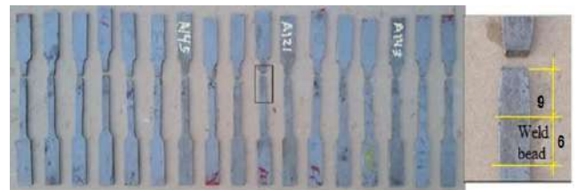
Fig. 9 - Breakage occurrence in HAZ: 9mm away from the bead.
