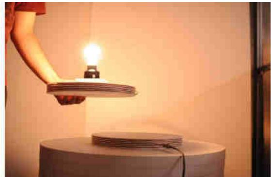
Fig.1: Wireless power transmission
