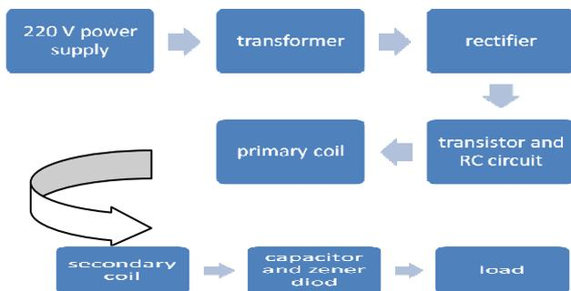
Fig.4:Block Diagram of Wireless Transmission
