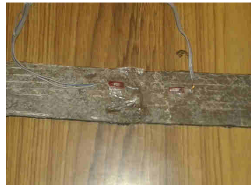
Fig.4.8: Installation of strain gauges
