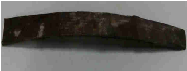
Fig4.3: Leaf spring of carbon fiber (out of fixture)
