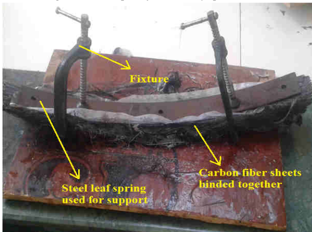
Fig4.2: Carbon fiber- leaf spring in fixture kept for drying
