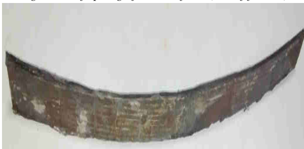
Fig.4.4: Leaf spring of carbon fiber (completely dried)
