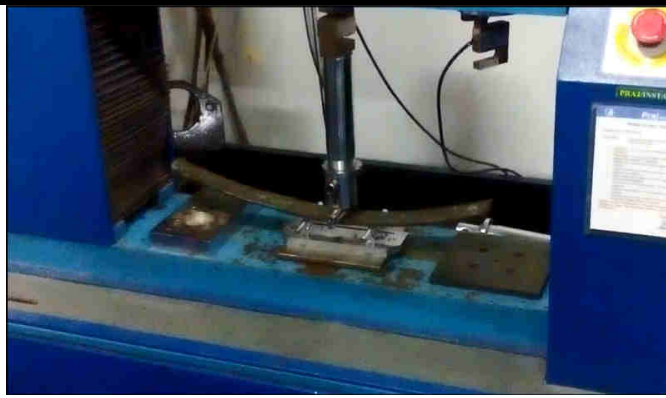
Fig.4.7: Experimental set up of leaf spring
