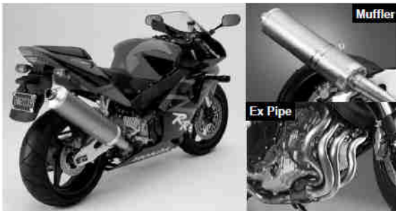
Fig.3: Application of Ti alloy in muffler and exhaust pipe
