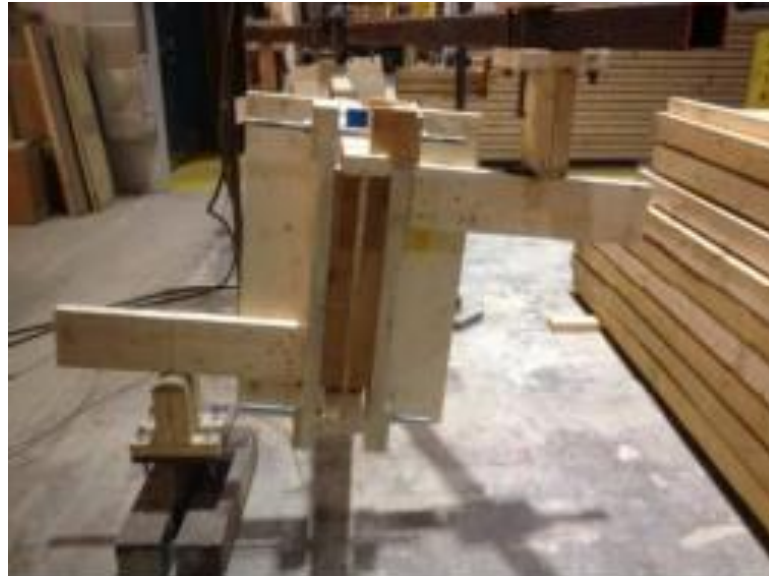
Fig. 2: I-Joist Torsional Rigidity Test Configuration for Whole I-Joist, Rémi St-Amour, Ghasan Doudak, 2017
