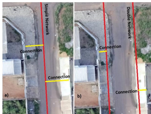
Fig.4: Connections outflowed in simple (a) and double network (b), showing the variation in the length of extensions
