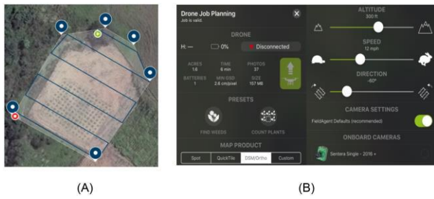
Fig. 2: Experimental area (A) and configuration of the FieldAgent™ system for UAV flight planning (B)
