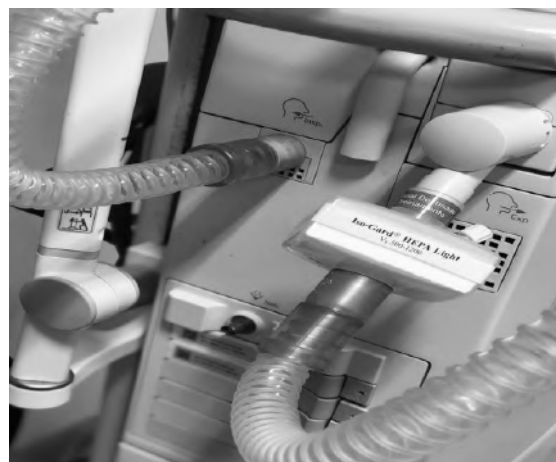
Fig.9: Positioning the HEPA filter in the expiratory circuit.
