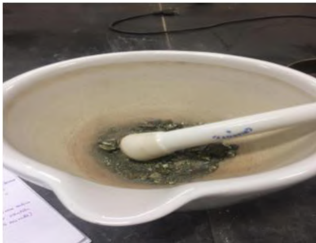
Fig. 4: Grinding of copper chalcopyrite ore in mortar and pestle
