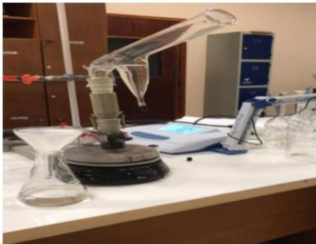
Fig. 7: Modified Hallimond tube of the laboratory type
