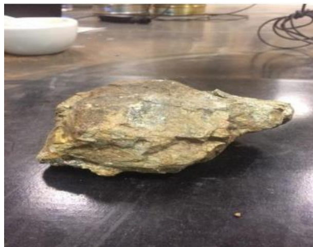
Fig. 2: Sulphide copper massif containing chalcopyrite
