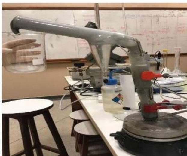
Fig. 8: Flotation being carried out in the modified Hallimond tube
