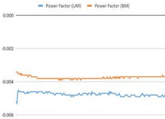
Fig 6. Comparative graph of the power factor of the System in Utility Model and in Back-up Mode using the datalogger
