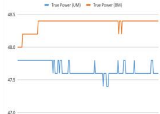
Fig 5. Comparative graph of the true power of the System in Utility Model and in Back-up Mode using the datalogger
