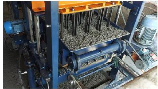
Figure 8. Pressing process for manufacturing the blocks.
