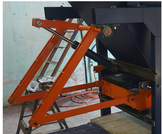
Fig.5: Pendulum mechanism of the drawer.
