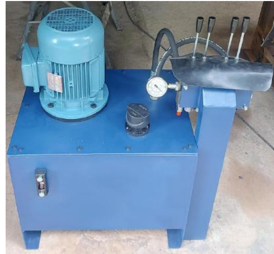
Fig.1. Hydraulic unit with valve block and levers.
