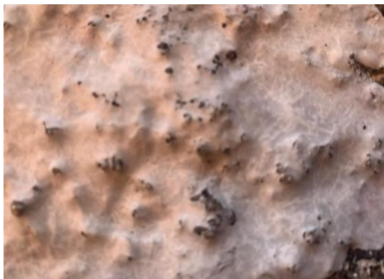
Fig 7. Tiner + Styrofoam + PVA Glue + Oil
