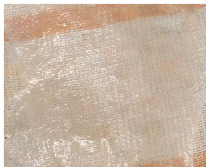
Fig2. Thinner and Styrofoam on fabric.
