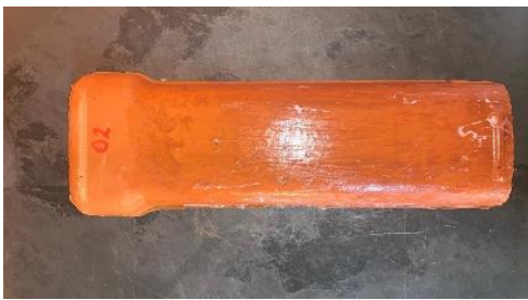
Fig 6. Thinner + Styrofoam + PVA glue Oil on the tile.
