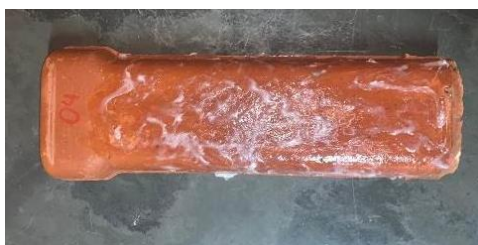
Fig 12. Thinner + Styrofoam + Fiberglass on the tile
