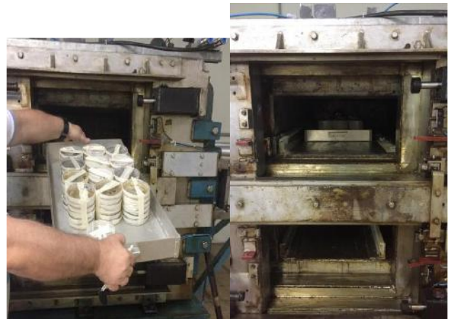
Fig. 3: Petri dishes inside the chambre of the irradiator
