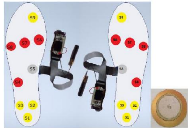
Fig. 7. Data acquisition/transmission and PFS sensor
