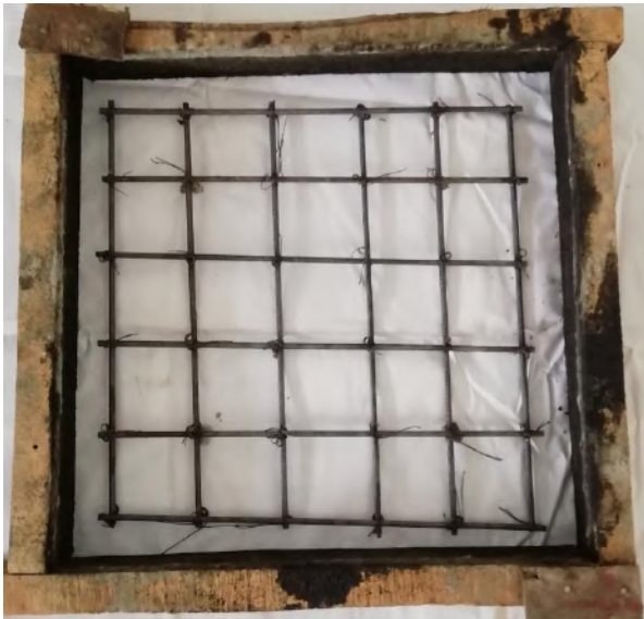
Fig.1: Reinforcement Details for Slab
