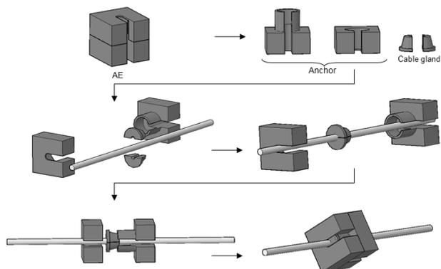
Fig. 7: Anchoring Elements applied to the cable
