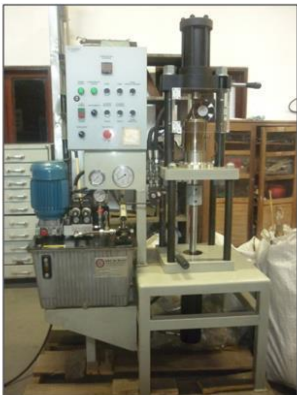
Fig. 1: Briquetting machine (Lippel- model LB-32) used in the study (Cellulose and Paper/Charcoal Laboratory/COTEI/INPA – Brazil).
