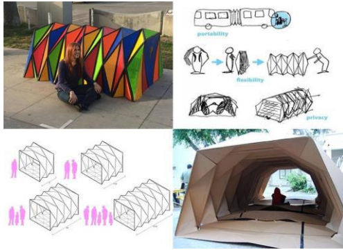
Fig.8: Sketches, perspective design and assembled structure of Cardborigami
