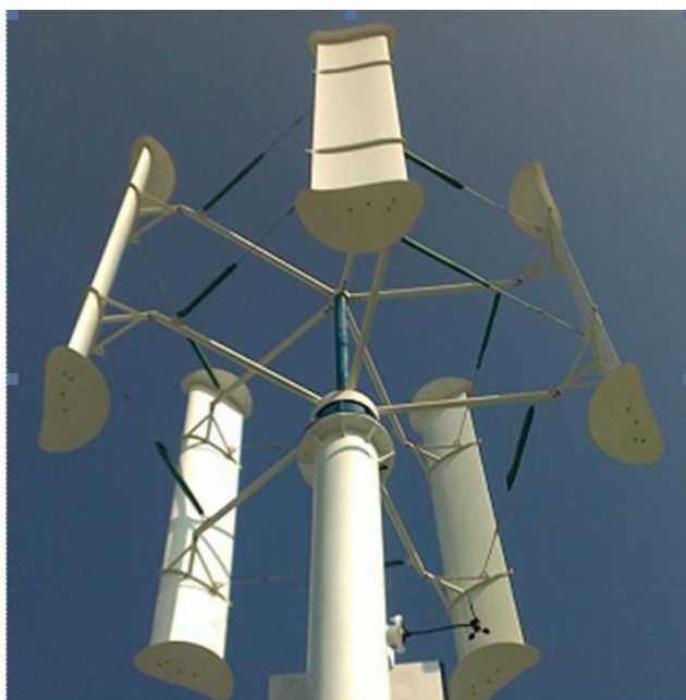
VAWT with relatively fixed blade angle
