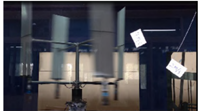
Wind tunnel test of VAWT with multiple disks structure
