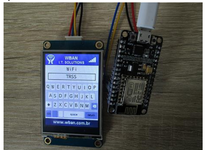
Fig. 10. The project in operation with the NodeMCU12e controller and with the display Nextion touchscreen [2].
