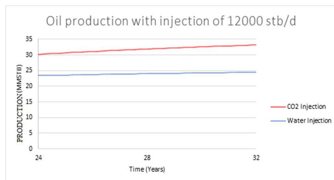
Fig.9: Oil production in the period of 24 to 32 years of simulation. Injection of 12,000 stb/d for all three methods.
