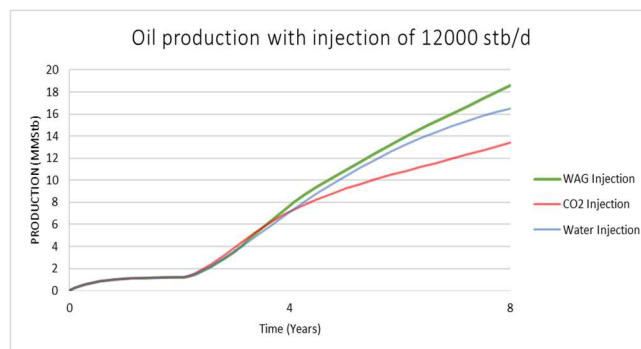
Fig.7: Oil production in the first 8 years of simulation with injection of 12,000 stb/d for the three methods.
