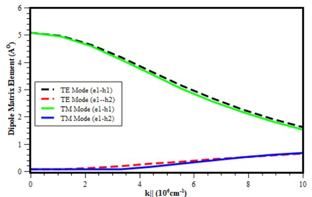
Fig.5. Behaviour of optical dipole matrix elements of designed  $Ga_{0.6}In_{0.4}P / Al_{0.3}Ga_{0.2}In_{0.5}P$  heterostructure
