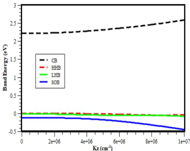
Fig.2. Bulk band structure diagram of compound material  $Al_{0.3}Ga_{0.2}In_{0.5}P$
