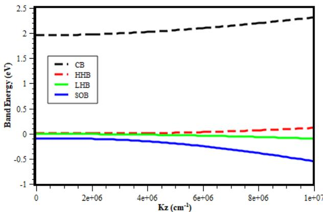
Fig 1. Bulk band structure diagram of compound material  $Ga_{0.6}In_{0.4}P$
