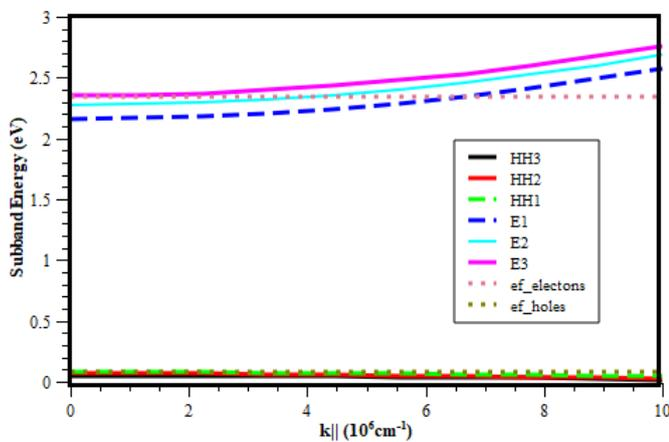
Fig.4. Energy dispersion  $Ga_{0.6}In_{0.4}P / Al_{0.3}Ga_{0.2}In_{0.5}P$  heterostructure
