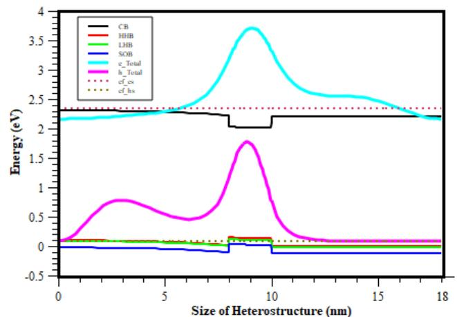
Fig.3. Electron and hole concentration  $Ga_{0.6}In_{0.4}P / Al_{0.3}Ga_{0.2}In_{0.5}P$  heterostructure
