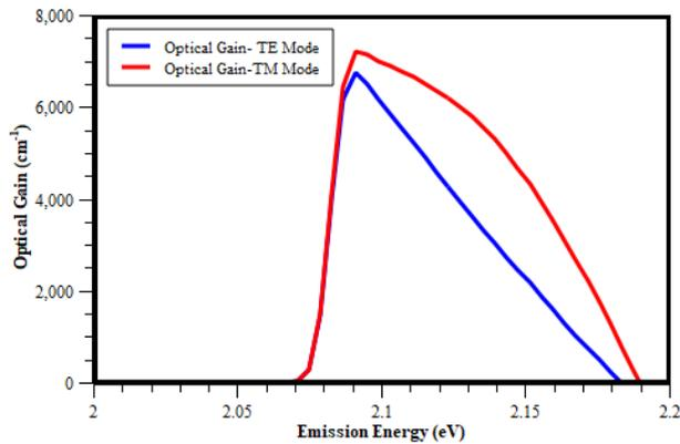
Fig. 6. Optical gain characteristic for designed  $Ga_{0.6}In_{0.4}P$  /  $Al_{0.3}Ga_{0.2}In_{0.5}P$  heterostructure
