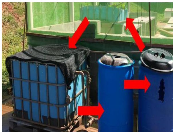
Fig. 4: Disposition of fish tank, decanter and sump tank.
