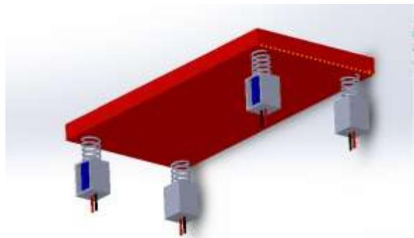
Fig.3: Isometric view of solenoid attached to entry carpets
