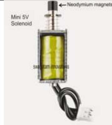
*Fig.5: Modified solenoid for generating electricity.*
