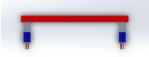
Fig.2: Front view of solenoid attached to entry carpets
