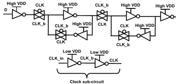
Figure 1: Typical transmission gate-based DFF topology driven by an LS clock
