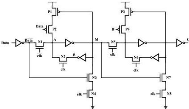
Figure 2: Proposed DFF topology that can reliably work with an LS clock signal whereas the data and output signals are at FS in Transistor level representation.
