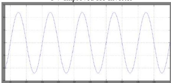
Fig. 7. (a) Simulink waveforms of the Grid Feeding Inverter Current
