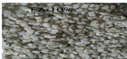
Fig. 5: The LLDPE - 90% + Flyash - 10% mixture.
