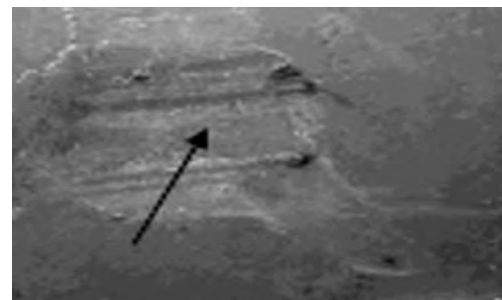
Fig.8: SEM Micrograph of damaged race way
