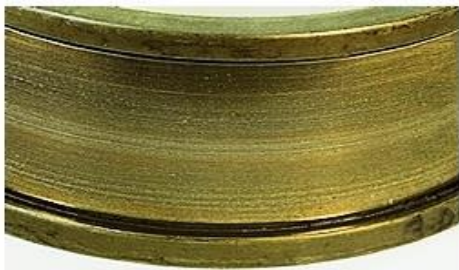
Fig.4: Discoloured Outer Ring of Roll Neck Bearings
