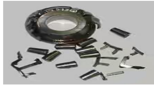
Fig.4: Damaged bearing in Wire Rod Mill
