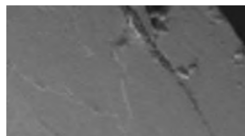
Fig.8: SEM Micrograph of damaged race way
